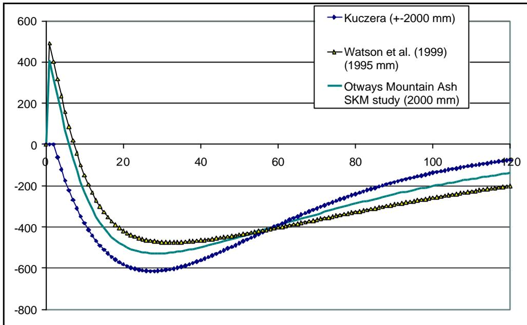
■ Figure 7-12 The stream flow response curve for Mountain Ash forest was fitted by eye to the two other curves shown in this Figure.
