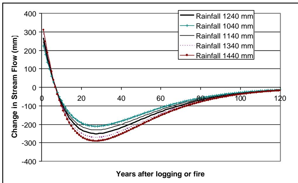
■ Figure 7-7 Adjustment of streamflow response curves for mean rainfall
