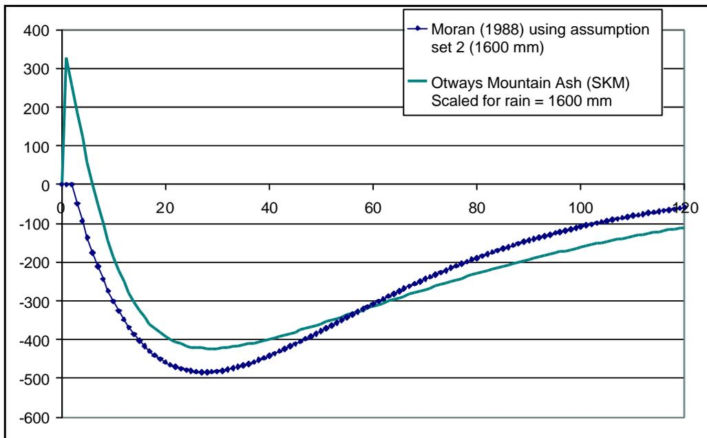
■ Figure 7-13 Comparison of the stream flow response curve for Mountain Ash forest used by Moran (1988) and used in this study. The curve shown in Fig. 2-4 has been scaled for a rainfall of 1600 mm.
